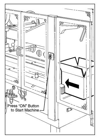
Figure 3-9 – Box Size Set-Up
